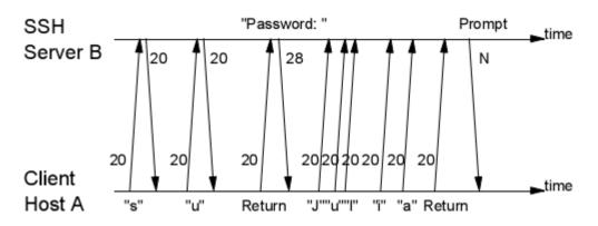
Figure 1. The illustration of timing attack scheme when user execute the su command.
